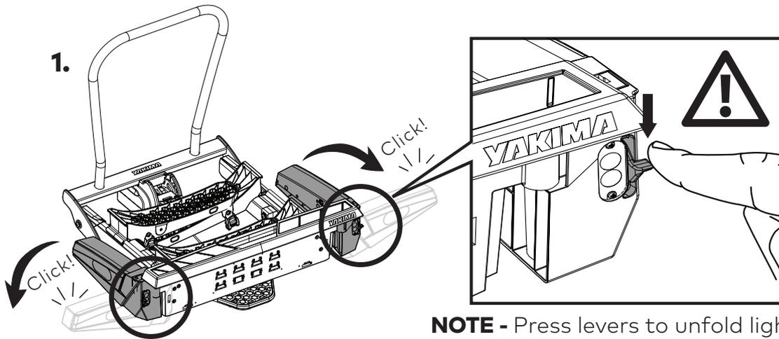
**NOTE** - Press levers to unfold lights
