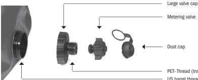
PET-Thread (Inner diameter 2,3cm/0.9in.) US barrel thread (Inner diameter 5,3cm/2.1in.)
