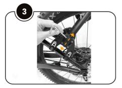
Depending on the size of your bike or seat, you can loosen the bolts shown above and slide the **spider rear rack** down to suit preferred height, and then tighten the bolts again.
